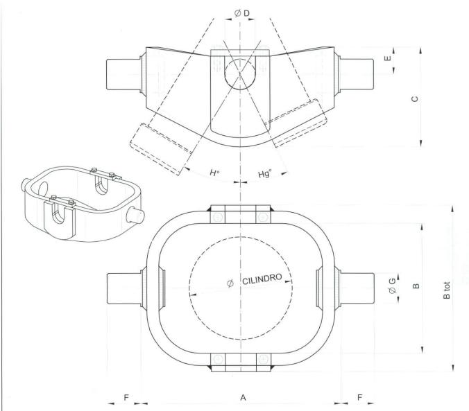
Materiale: Acciaio Fe 430/C - Material: Steel Fe 430/C - Materiau: Acier Fe 430/C - Verkstoff: Prepstahl Fe 430/C
